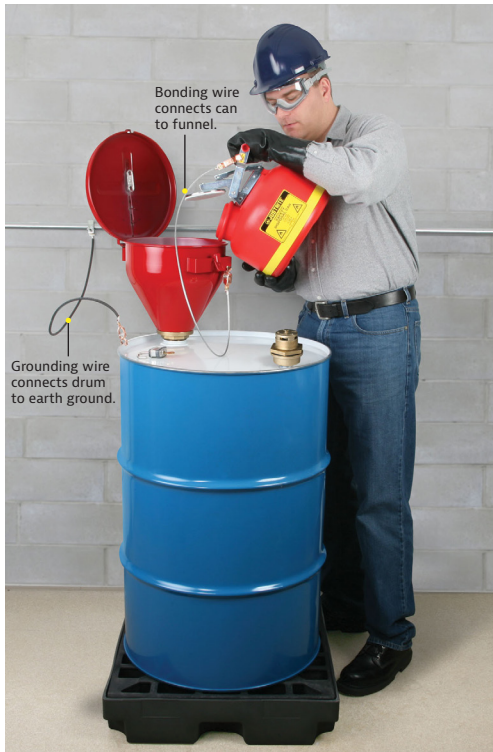
Use bonding wire while pouring liquids into other containers.
