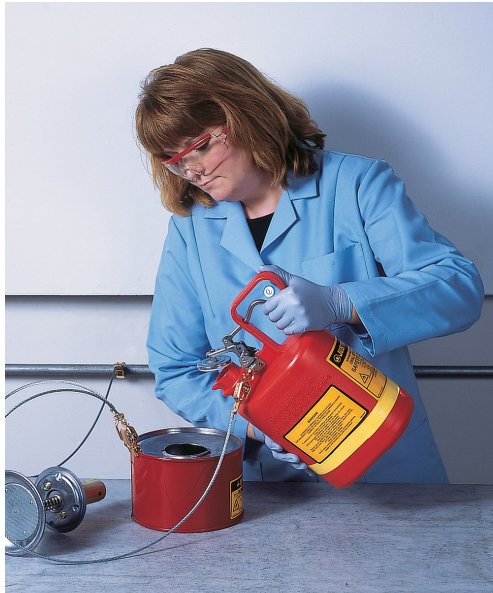
To properly ground when using nonmetallic containers, an antistatic wire connects the poly can's cover assembly (with special internal insert) to the receiving vessel. A second antistatic wire connects the receiving vessel to a ground pipe.
