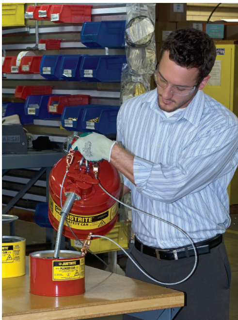
Antistatic wires with alligator clips are a popular choice when grounding containers. Clips with their sharp teeth can be "wiggled" to ensure metal to metal contact on painted surfaces.
