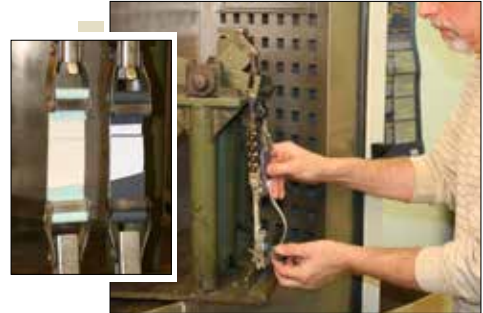
Dead load seam shear test
