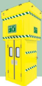
Designed for severely cold climates, polar tank showers incorporate a double-skinned fiberglass insulated cubicle to protect the user from the elements. Double swing push open doors provide unimpeded access and protection from the elements. Windows in the doors enable the casualty to be monitored while using the emergency safety shower in case assistance is required. Room heater maintains the internal cubicle temperature.
