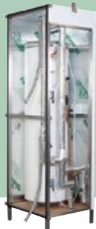
Developed to supply tepid water to emergency safety showers and eye wash units located in extreme freezing conditions, heated water tanks are available in a 119 US gallon (450 liter) capacity. Insulated with polyurethane and encased in a GRP-clad stainless steel frame, these units supply heated water to one or more emergency showers so that they also meet the temperature and duration criteria in the ANSI standard.
