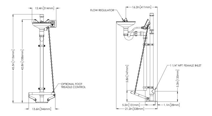
VARIATIONS IN MANUFACTURING AND ASSEMBLY ALLOW FOR  $\pm 1/8$  IN [3MM] PER THREADED JOINT.
