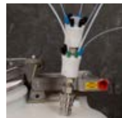
Manifold 28177 with stacker 28179 and tubing connectors 28188 and 28189.
