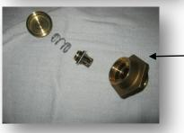
3) Cap, spring, valve assembly, & flange sequence
