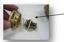
2) Assembly is spring loaded, use care with parts as you unassembled them
