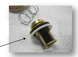
4) Valve subassembly as assembled
