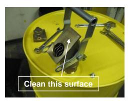
2) You can now relax the handle. This is a view of the valve unassembled. It is a good idea to clean the brass slide surface clear of grime before installing the new gasket. If there are, any gouges in the brass slide surface replace the entire faucet.
