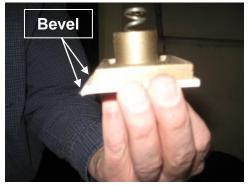
3) Make sure you seat the "brass gasket pad bearing-plate" into the inset of your new "PTFE gasket pad". Orient both bevels in the same direction (as shown).
