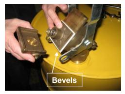
4) Orient the "brass positioning-plate", "bearing-plate", "PTFE gasket pad" and "compression spring" as shown left and below. Note: how the specific geometry is orientated for each part in the picture (both bevels are opposite of the handle's grip).
