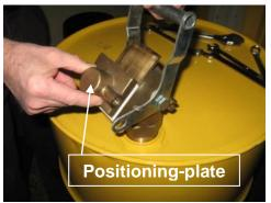
5) Again, this step is a two-person job. With one person holding the spring loaded handle; have them position the handle at a location convenient for the other person to reinstall the shoulder bolts. With one hand compress down the spring loaded brasspositioning plate while using the other hand to insert and tighten the shoulder bolt. Then move to the other side.
