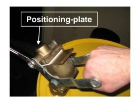
1) This step is a two-person job. One person should hold the spring loaded handle while the other use a 3/4" wrench to remove the two shoulder bolts that secure the "brass positioning-plate".
