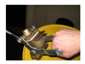
7) Once both shoulder bolts are secure, tighten them both with a 3/4" wrench. Check to make sure the gate valve opens and closes freely with the handle. If it works fine, you can install the faucet on a drum, and if it does not leak, you have done a good job. Please, verify your work.
